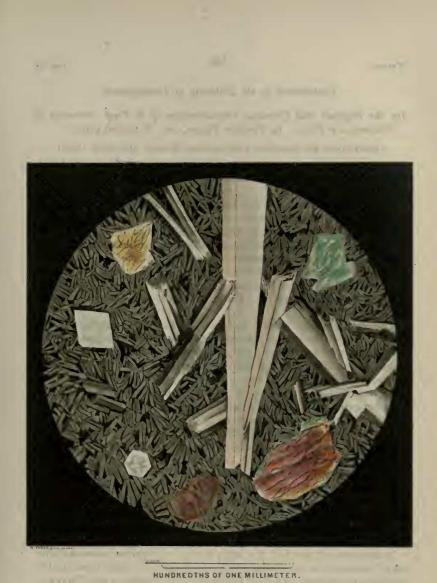
Thin section of Trap from Williamson's Point, Lancaster Co.Pa. Magnified 400 Diameters.
